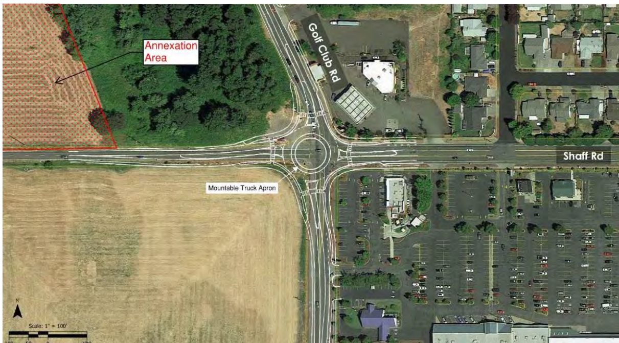
Figure 3. Proposed Round About at intersection of Shaff Rd and Golf Club Rd.
